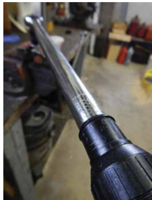
Each was torqued with a torque wrench to pre set 35 lbs.
