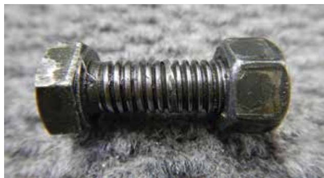
Here is the bolt that was pre-sprayed then over torqued, which resulted in the nut over tightening and destroying the threads.
