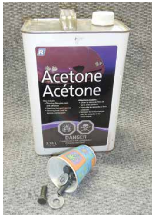
All of the hardware was washed in acetone and let dry to strip off all oil.
