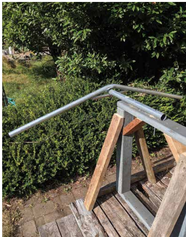
A bent pipe on a second hoop bender, again mounted to a deck. This bender was designed for the sides of the high tunnel frame.
