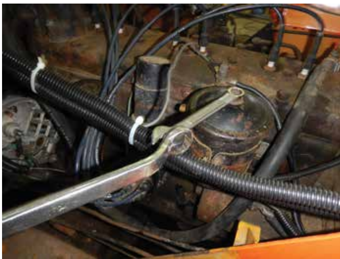
Not needed in this case but a great trick to know, doubling a box end wrench onto an open end for tight places and higher torque, here is removing the oil canister lid bolt
