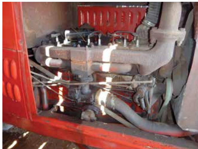
'IL6' in the MH101 shows the up draft carburetor (on the bottom) and the up swept front exhaust; also shown is the governor (belt driven at the front this of the engine).
