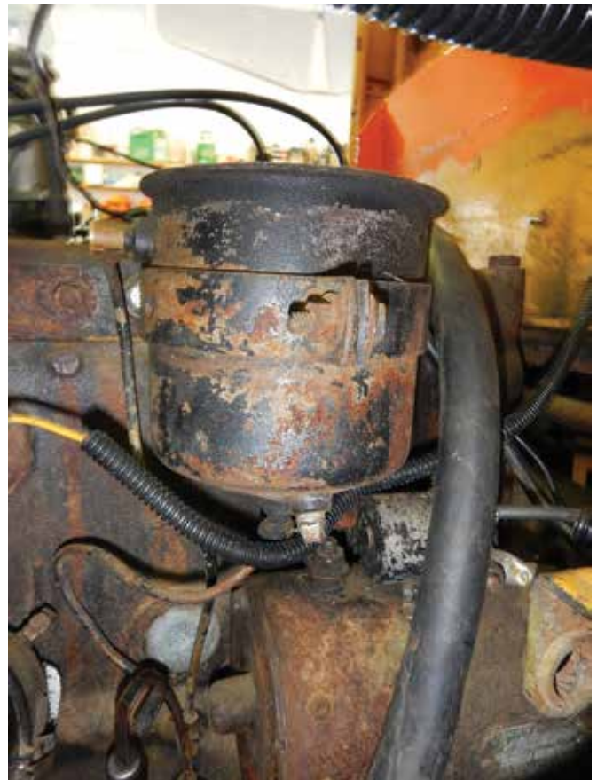
The oil canister on the opposite side with the silver bung shown at the bottom centre (note the anti chaff wrap on the wiring)
