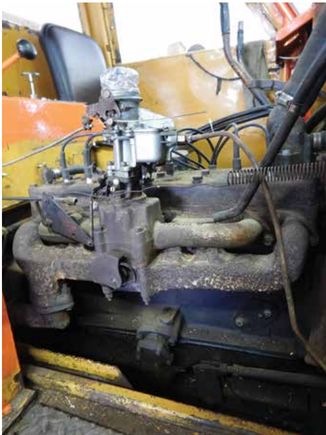
'IL6' in the Muskeg shows the down draft carburetor (on top) and down swept rear exhaust; the mechanical fuel pump on this side at front has been removed.
