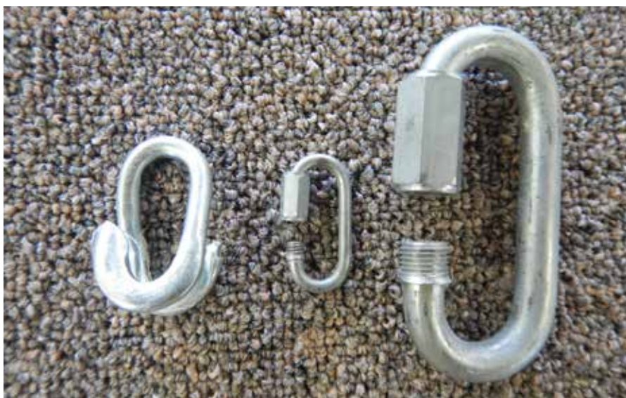
Left is a link replacer which replaces the broken link and is then hammered flat. Quick links (threaded) come in a wide selection of sizes and are quick and easy to use
